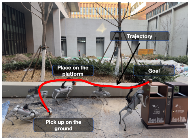
Fig.7: Long-horizon trajectory tracking. The robot can switch between locomotion and manipulation to track the target end-effector pose.
